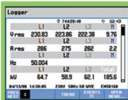
Logging function allows you to customize measurement selections and provides analysis of user-selectable parameters to find intermittent problems or relate PQ issues to other phenomena/events.
