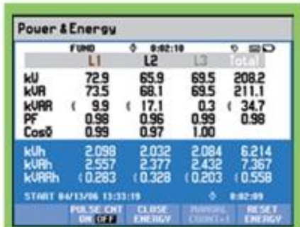
Measure and record power (W), VA and VARs. The Fluke 434/PWR adds the ability to record energy consumption
