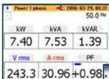
Equipment performance measurement - power consumed by single- and three-phase balanced loads.
