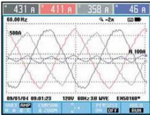
Scope view shows voltage and current waveforms for three phase installations. You can toggle to a phasor diagram at any time.
