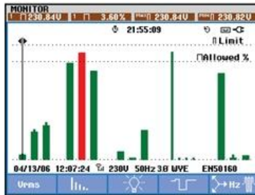
The System-Monitor overview screen gives instant insight into whether the voltage, harmonics, flicker, frequency and the number of dips and swells fall outside the set limits.
